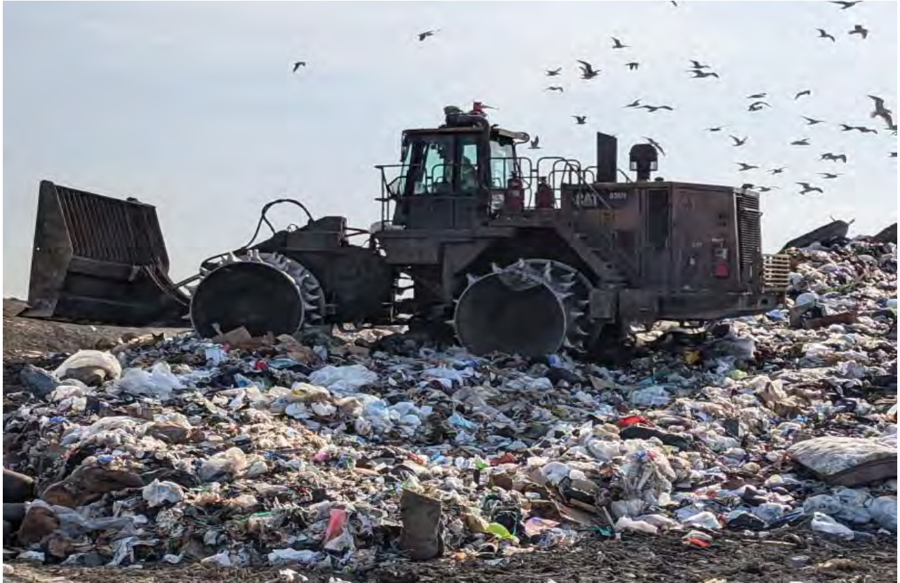
Example of good compaction in working face
